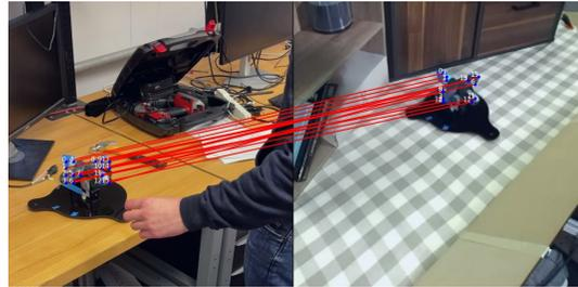
Figure 8. Valve Rotation Human Demo vs Robot Rollout: Domain Gaps and Point Matches.
